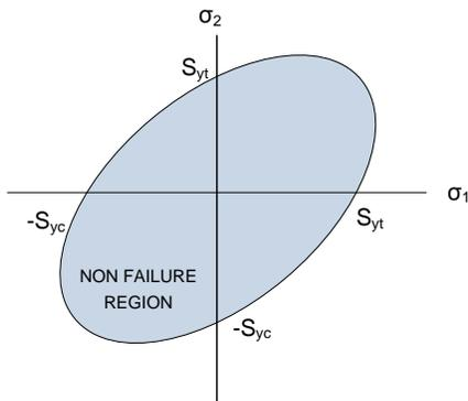
Ductile Loading: Distortion Energy Theory
